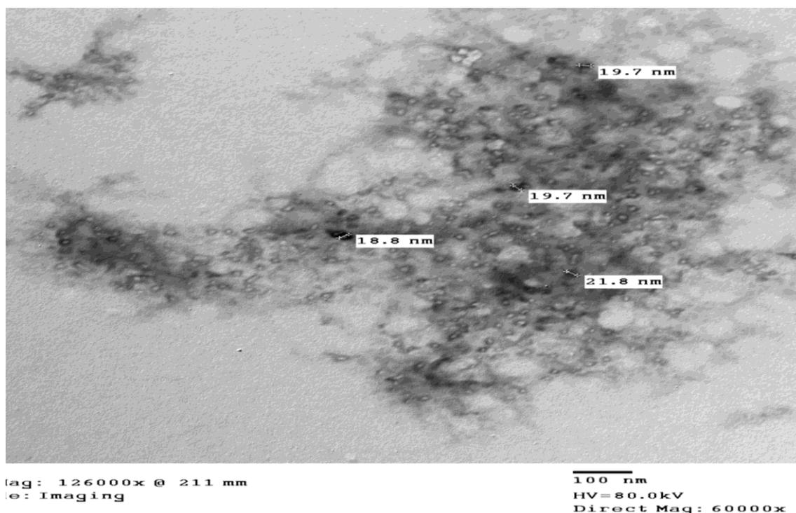
**Figure 1.** Transmission electron microscopy micrograph of chitosan nanoparticles
